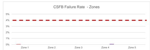
**CSFB Failure Rate** represents the ratio between unsuccessful fall back attempt to lower technology than 4G (LTE) and all calls made (both successful & unsuccessful). When there is 4G (LTE) present before starting the session.
