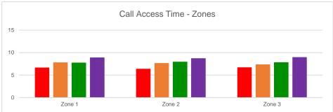
**Call Access** represents the period of time elapsed from the sending of a complete destination address (target number) to the setting up of a call to the receiving terminal.
