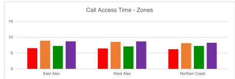
**Call Access Time** represents the period of time elapsed from the sending of a complete destination address (target number) to the setting up of a call to the receiving terminal.
